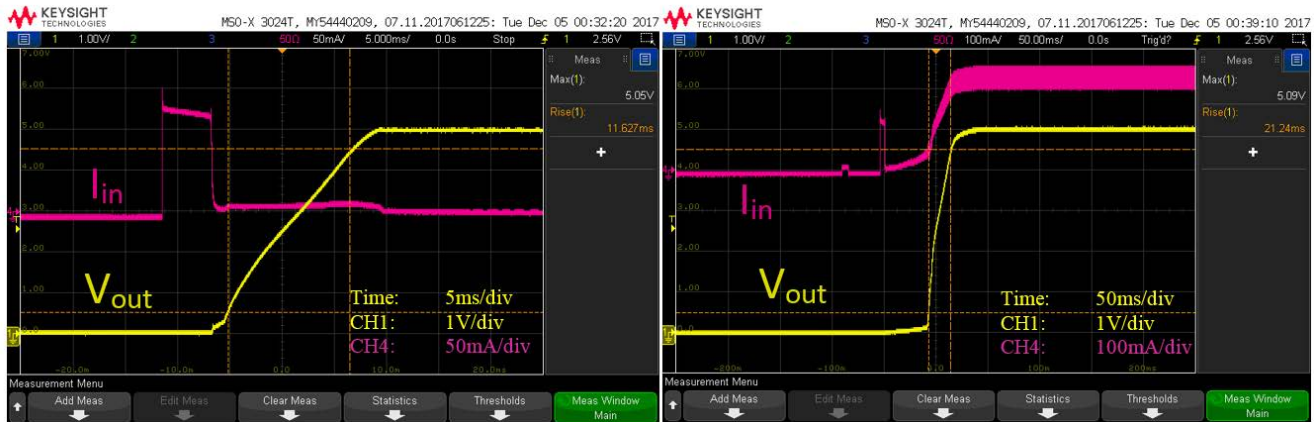
Figure 8.1. Si3406-Non-Isolated Flyback C3 EVB Input Current and Output Voltage Soft-Start at Low Load (Left) and Heavy Load (Right) Conditions
