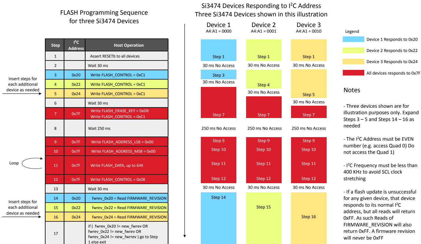
Figure 2.15. Flash Loading Sequence
