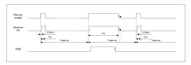
Bit 0 (en): Enables the Low Duty-Cycle Mode. Wake-up timer interrupt not generated in this mode.
