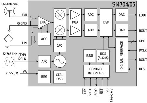
Figure 7. Functional Block Diagram
