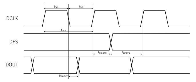
Figure 6. Digital Audio Interface Timing Parameters, I<sup>2</sup>S Mode
