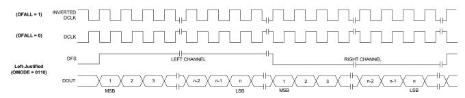
Figure 10. Left-Justified Digital Audio Format
