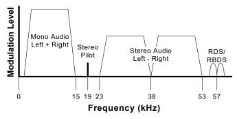
Figure 8. MPX Signal Spectrum
