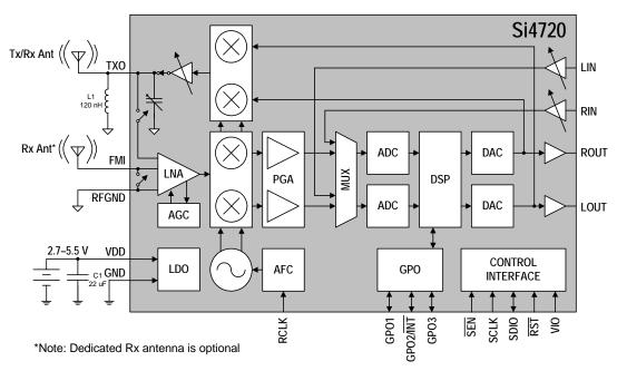
Figure 14. Functional Block Diagram
