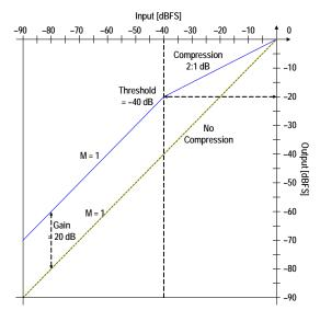
Figure 24. Audio Dynamic Range Transfer Function
