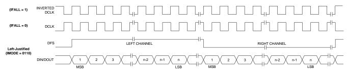
Figure 22. Left-Justified Digital Audio Format
