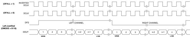
Figure 17. Left-Justified Digital Audio Format
