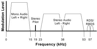
Figure 19. MPX Signal Spectrum
