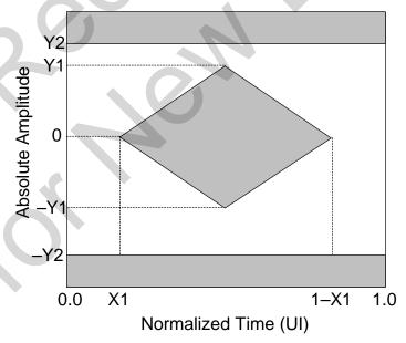
Figure 5. Transmitter Differential Input Mask (TD)
