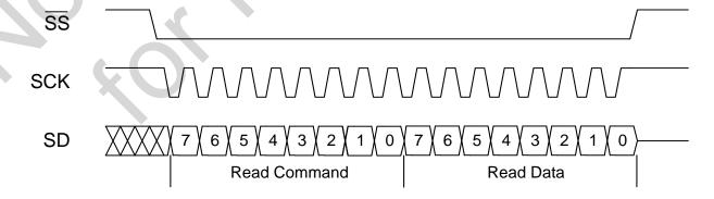
Figure 8. SPI-Like Interface Read Command
