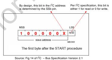
Figure 22. Device I<sup>2</sup>C Address
