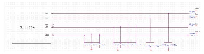
Figure 11. Recommended of Si53106 Power Filtering
