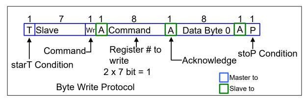
Figure 8. Byte Write Protocol
