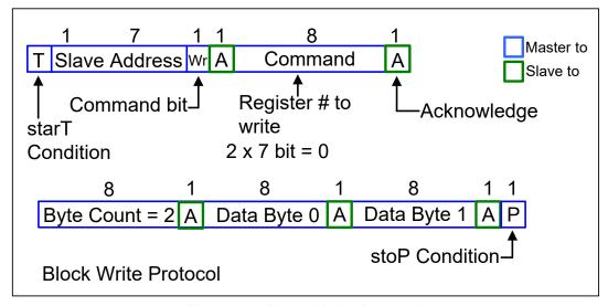
Figure 10. Block Write Protocol
