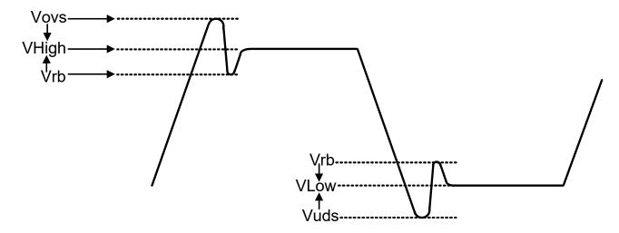
Figure 4. Single-Ended Measurement Points for  $V_{ovs}, V_{uds}, V_{rb}$
