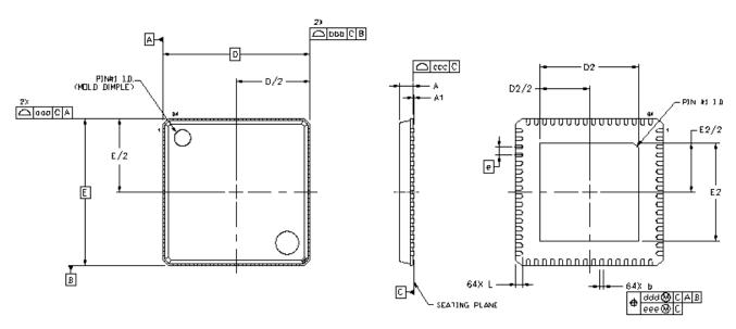
Figure 12. 64-Pin Quad Flat No Lead (QFN) Package
