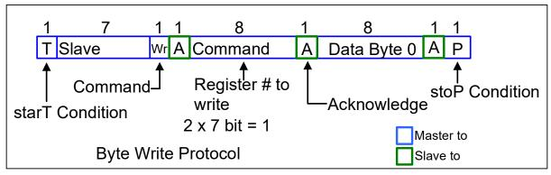
Figure 8. Byte Write Protocol
