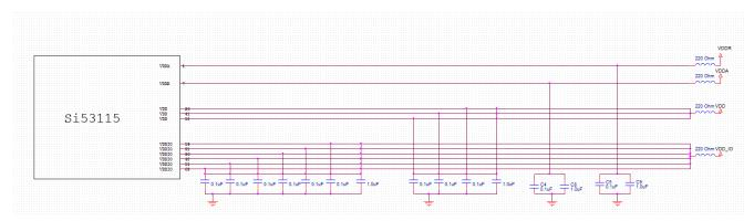
Figure 11. Recommended Si53115 Power Filtering
