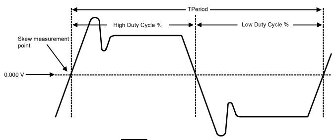
Figure 5. Differential (CLOCK–CLOCK) Measurement Points (T<sub>period</sub>, Duty Cycle, Jitter)
