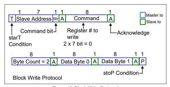
Figure 10. Block Write Protocol
