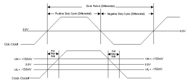
Figure 2. Differential Output Signals (for AC Parameters Measurement)
