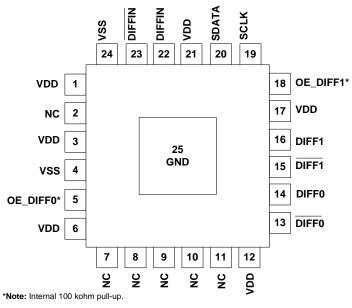
Figure 4. 24-Pin QFN
