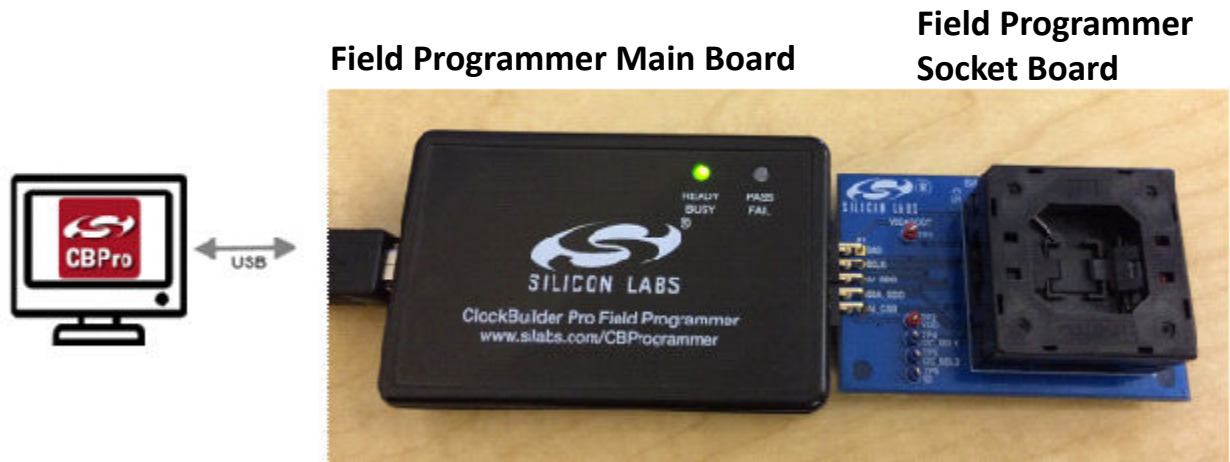
Figure 4.3. System from PC to Programming CBPROG-DONGLE Board to Field Programmer Socket Board
