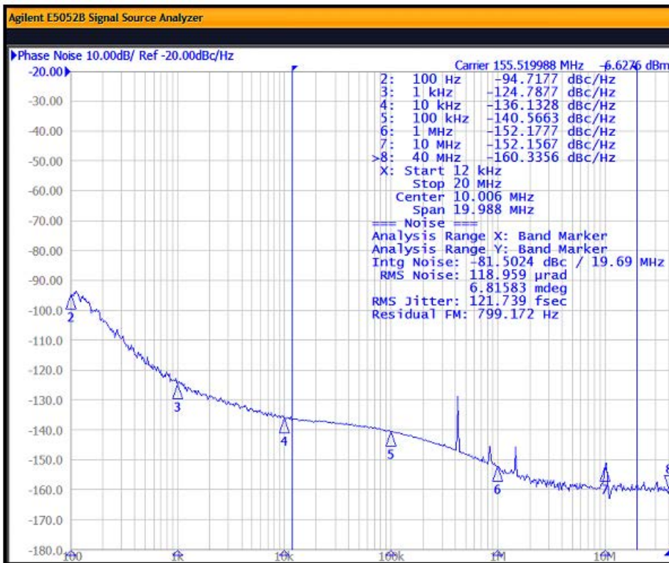
Figure 8.3. Input = 25 MHz; Output = 155.52 MHz, 2.5 V LVDS
