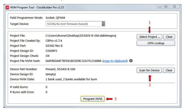
Figure 4.9. Programming In-socket, Non-Firmware Based Devices
