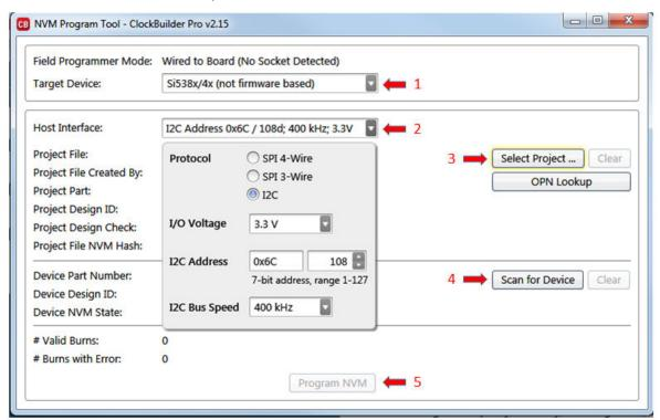
Figure 4.19. Programming In-system, Non-firmware Based Devices
