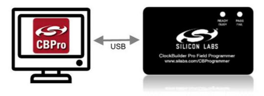
Figure 4.11. PC to CBPROG-DONGLE Connection
