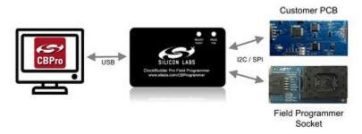
Figure 4.1. PC to CBPROG-DONGLE Connection
