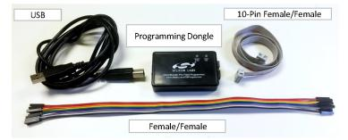
Figure 1.2. CBPROG-DONGLE Kit Contents
