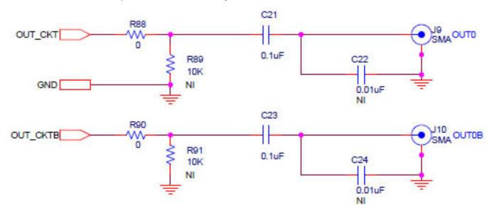
Figure 7.1. OUtput Clock Termination Circuit
