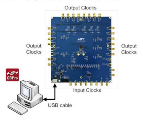
Figure 9.1. EVB Connection Diagram
