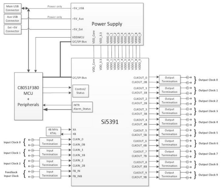
Figure 1.1. Si5391P-A EB Functional Block Diagram
