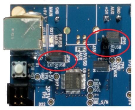
Figure 9.2. JP15-JP16 Standard Jumper Shunt Installation
