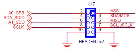
Figure 12.1. Serial Communications Header J17
