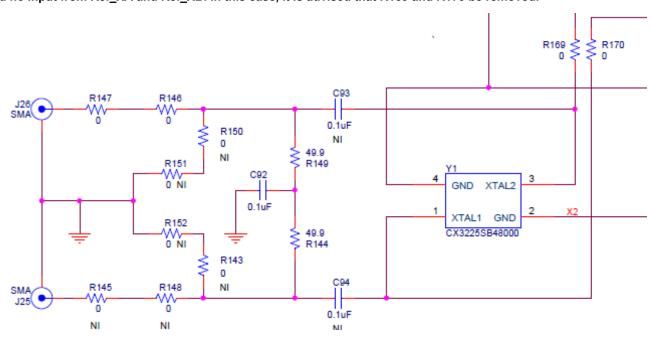
Figure 6.1. External Reference Input Circuit
