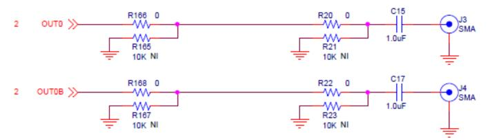
Figure 8.1. Output Clock Termination Circuit
