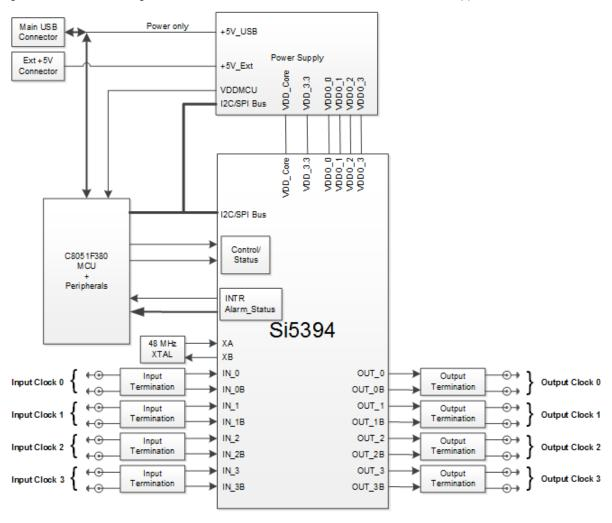
Figure 1.1. Si5394 EVB Functional Block Diagram
