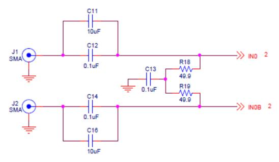
Figure 7.1. Input Clock Termination Circuit
