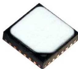
Figure 8. Si7005 with Factory-Installed Protective Cover
