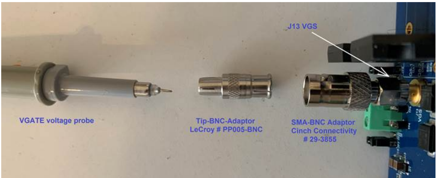
Figure 2.6. Connection for VGS Scope Probe at J13
