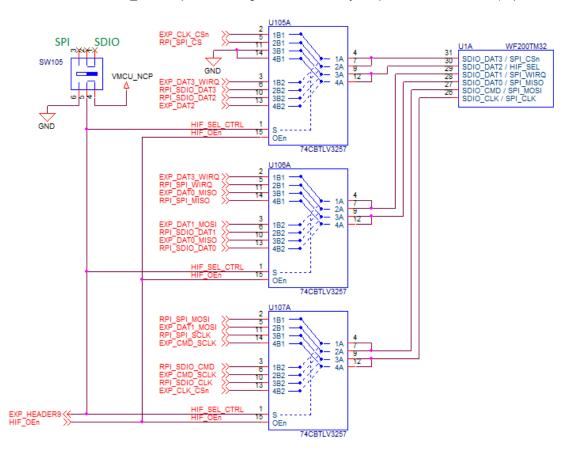
Figure 3.1. Host Interface Multiplexer Circuit
