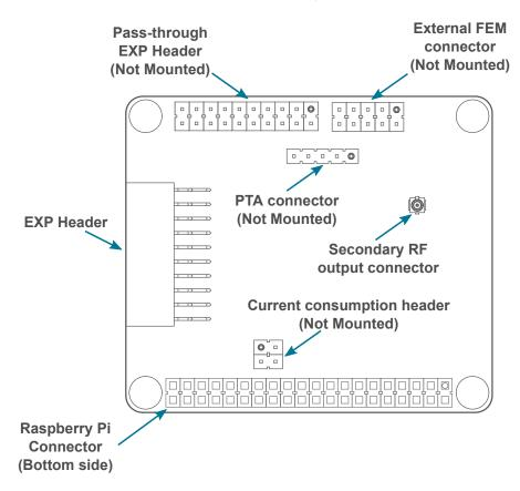
Figure 4.1. WF200 Wi-Fi Expansion Kit Connector Layout
