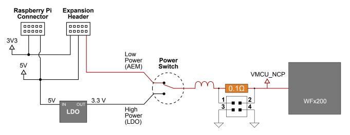
Figure 4.6. WF200 Wi-Fi Expansion Kit Power Topology
