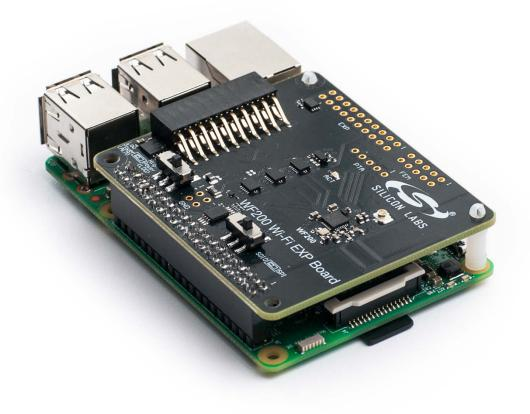
Figure 1.2. WF200 Wi-Fi Expansion Kit Connected to a Raspberry Pi and Secured With Nylon Standoffs
