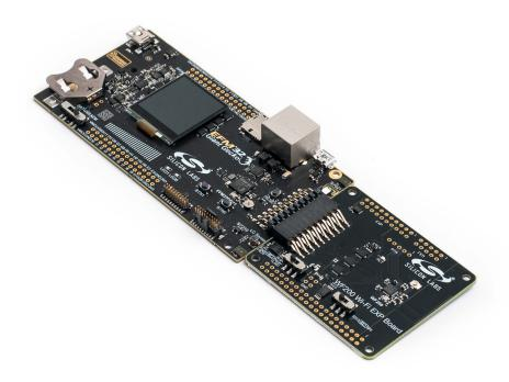
Figure 1.1. WF200 Wi-Fi Expansion Kit Connected to a Silicon Labs EFM32GG11 MCU STK
