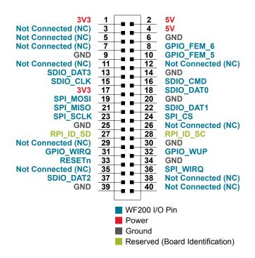
Figure 4.3. Raspberry Pi Connector
