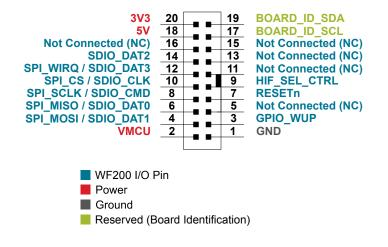
Figure 4.2. Expansion Header
