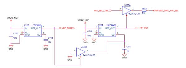
Figure 3.2. Power-on and Manual Reset Circuit Diagram
