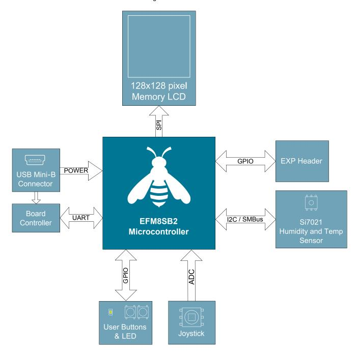
Figure 2.1. EFM8SB2-SLSTK2011A Block Diagram
