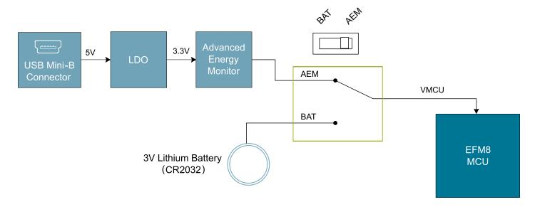
Figure 4.1. EFM8SB2-SLSTK2011A Power Switch
