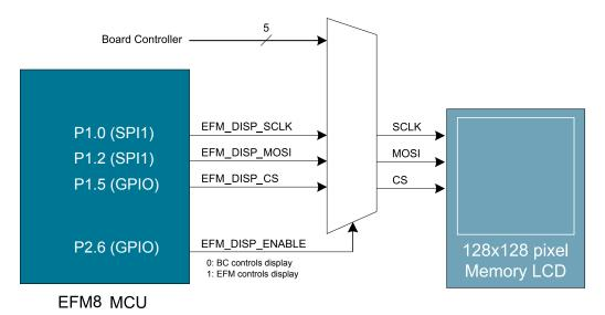
Figure 5.3. 128x128 Pixel Memory LCD
