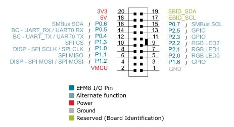
Figure 6.2. Expansion Header
