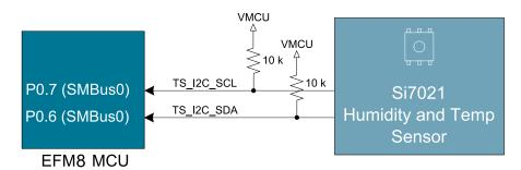
Figure 5.4. Humidity and Temperature Sensor
