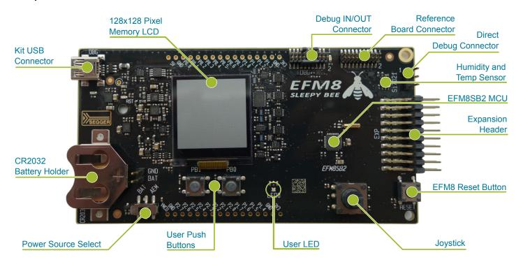
Figure 3.1. EFM8SB2-SLSTK2011A Hardware Layout
