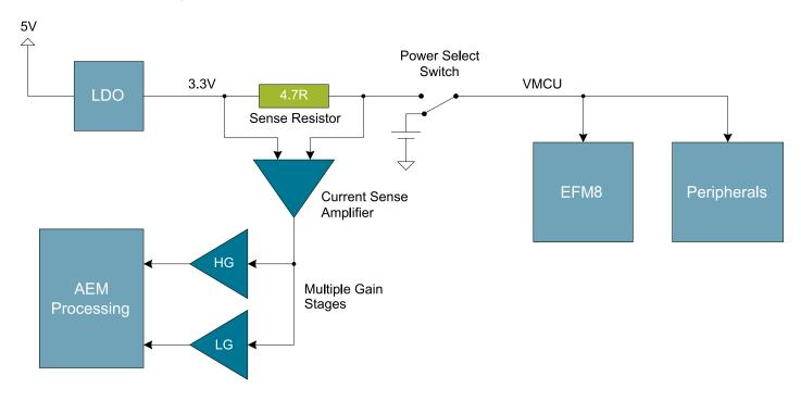
Figure 8.1. Measuring EFM8SB2-SLSTK2011A Current Using AEM
