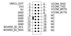
Figure 6.5. Reference Board Header
