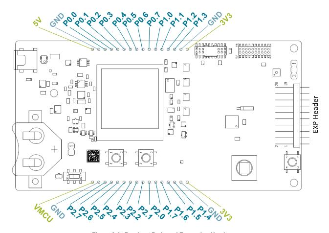
Figure 6.1. Breakout Pads and Expansion Header
