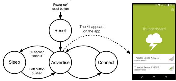
Figure 2.1. Kit Firmware State Diagram and App Start-up Screen
