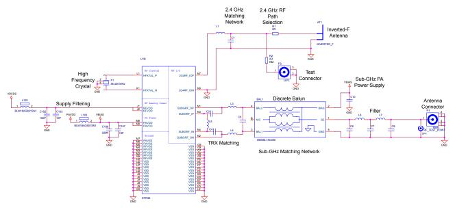
Figure 4.1. Schematic of the RF Section of the BRD4254A
