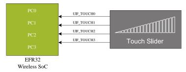
Figure 3.2. Touch Slider Pin Mapping
