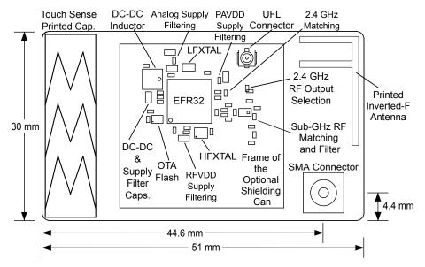
Figure 5.1. BRD4254A Top View
