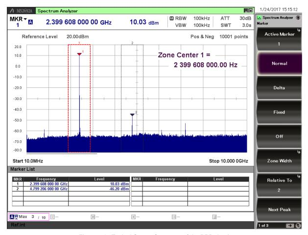
Figure 7.2. Typical Output Spectrum of the BRD4254A
