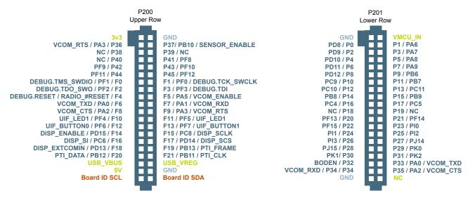
Figure 2.1. BRD4254A Radio Board Connector Pin Mapping
