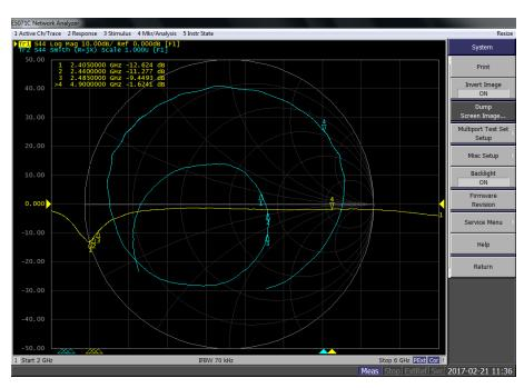
Figure 4.2. Impedance and Reflection of the Inverted-F Antenna of the BRD4254A Board Measured from the Matching Output
