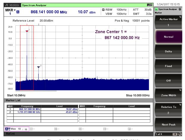
Figure 7.1. Typical Output Spectrum of the BRD4254A
