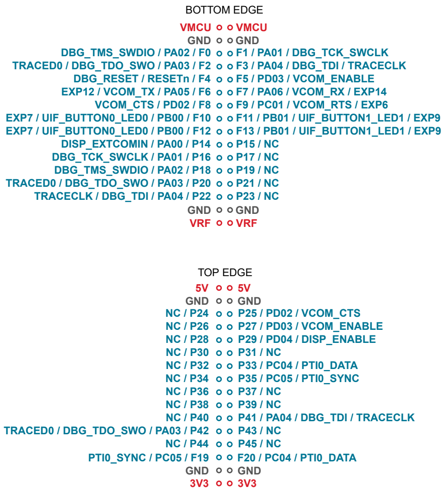
Figure 3.3. Wireless Pro Kit Mainboard (BRD4002A) Breakout Pad Pin Mapping
