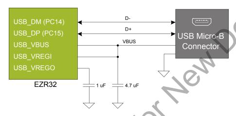
Figure 5.1. Radio Board USB Connector
