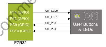
Figure 5.2. Buttons and LEDs
