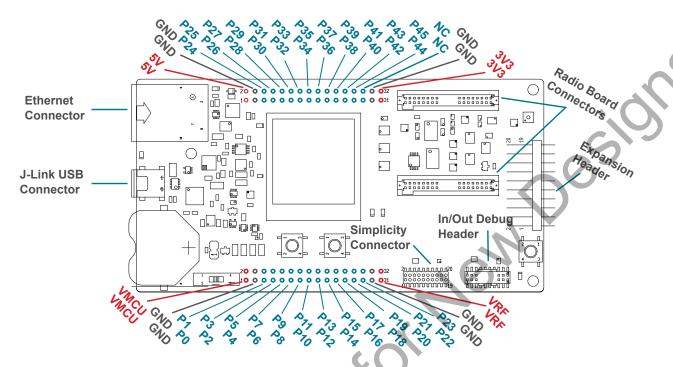
Figure 3.1. Mainboard Connector Layout
