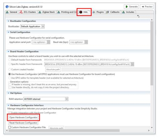
Figure 3.1. Open Hardware Configurator
