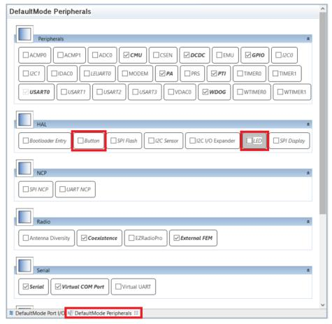
Figure 3.2. Disable Button and LED Configurations
