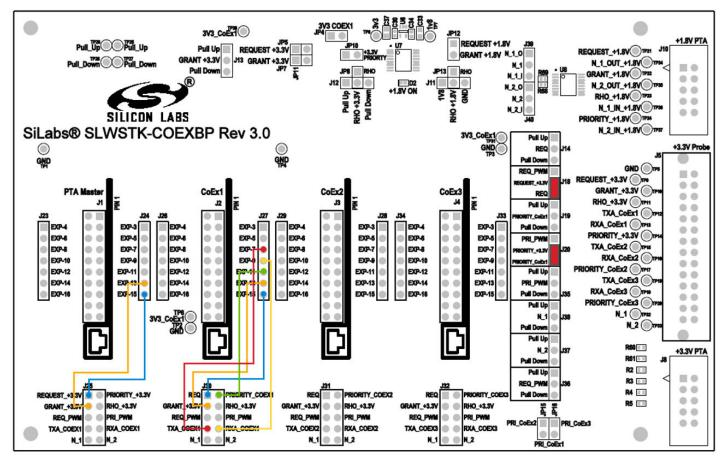
Figure 3.4. Coexistence Backplane Board Jumpers for Single-EFR32 Radio
