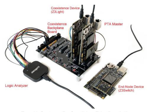
Figure 1.2. Coexistence Test Setup Using a Zigbee Example (1)
