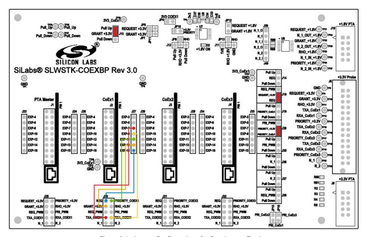
Figure 2.4. Jumper Configurations for Coexistence Testing
