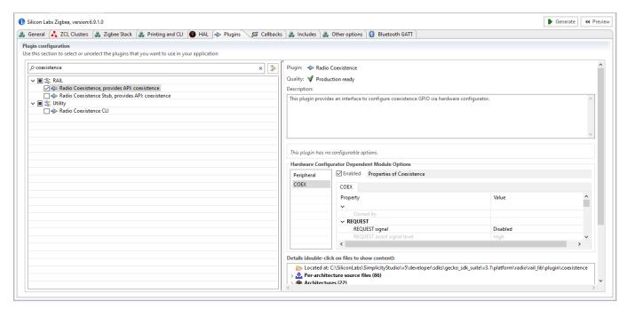
Figure 2.2. Enabling the Coexistence Configuration Plugin
