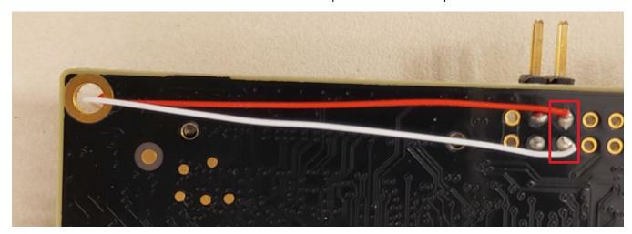
Figure 3.15. PTI Header Soldering
