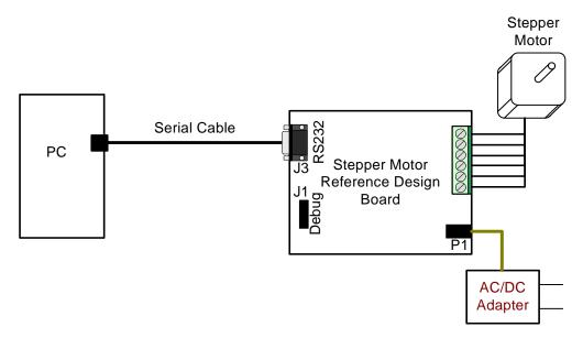
Figure 3. Stepper Motor Reference Design Terminal Setup
