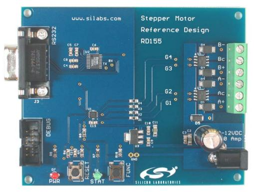
Figure 1. Stepper Motor Reference Design Board
