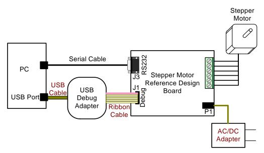
Figure 7. Development Setup using the USB Debug Adapter
