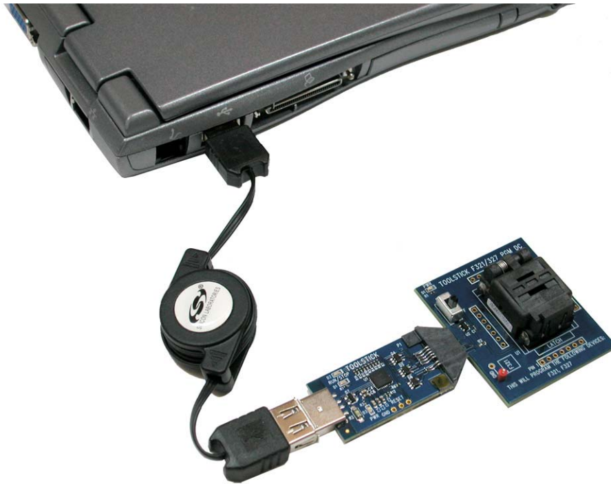
Figure 5. ToolStick Socket Platform Connected to PC
