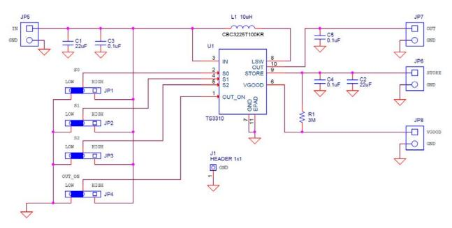
Figure 2.1. TS331x-EVB Schematic
