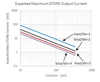
Figure 2.3. Expected Maximum STORE Output Current with 85% Efficiency vs. Inductor Value
