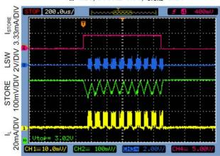
STORE Output Voltage Ripple, Inductor Current, and LSW Voltage : Circuit A V<sub>IN</sub>=1.2V, STORE=3V, I<sub>STORE</sub>=10mA
