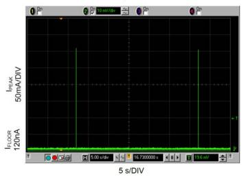
Input Quiescent Current : Circuit A with No-Load V<sub>IN</sub>=3V, STORE=3V
