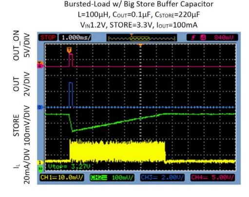
Figure 2.8. 220 µF C<sub>STORE</sub> Recovery Scope Capture
