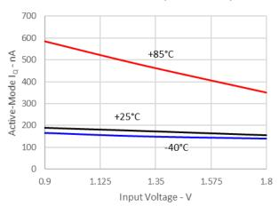
Active-Mode  $I_Q$  vs Input Voltage with No Load : Circuit B (STORE=1.8V)
