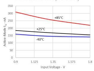
Active-Mode I<sub>Q</sub> vs Input Voltage with No Load : Circuit A (STORE=3V)
