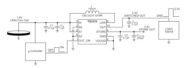
Figure 2.7. Bursted Load Application Circuit
