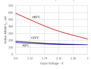
Active-Mode I<sub>Q</sub> vs Input Voltage with No Load : Circuit A (STORE=5V)
