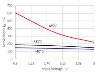
Active-Mode I<sub>Q</sub> vs Input Voltage with No Load : Circuit B (STORE=3V)
