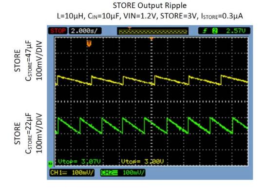
Figure 2.6. Output Voltage Ripple Comparison
