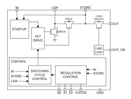
Figure 2.1. TS331x Functional Block Diagram
