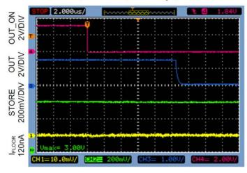
Short STORE to GND for 1msec Recovery : Circuit A  $V_{\text{IN}}$ =1.2V, STORE=3V,  $I_{\text{STORE}}$ =2mA
