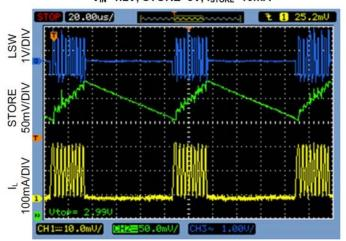
STORE Output Voltage Ripple, Inductor Current, and LSW Voltage : Circuit A V<sub>IN</sub>=1.2V, STORE=3V, I<sub>STORE(MAX)</sub>=35mA
