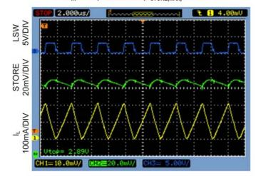
Startup : Circuit A with  $R_{\text{IN}}{=}10\Omega$   $V_{\text{IN}}{=}0.9V,$  STORE=1.8V,  $I_{\text{STORE}}{=}0.18\mu\text{A}$
