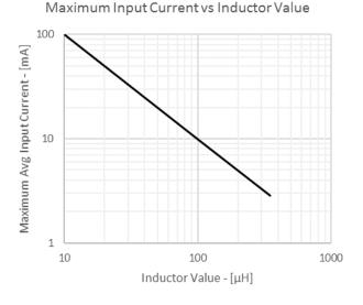
Figure 2.4. I<sub>IN(AVG,MAX)</sub> vs. Inductor Value
