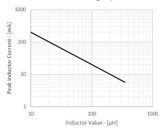
Figure 2.5. Inductor Peak Current vs. Inductor Value
