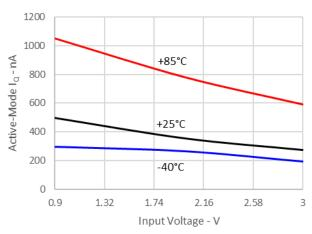
Active-Mode I<sub>Q</sub> vs Input Voltage with No Load : Circuit B (STORE=5V)
