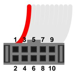
Figure 2. 32-Bit USB Debug Adapter Connector
