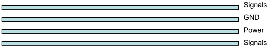
Figure 17: Typical 4-layer PCB construction
