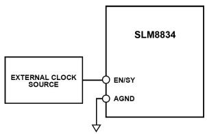
Figure 13. Synchronize to an External Clock
