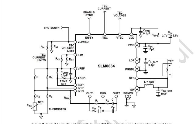
Figure 2. Typical Application Circuit with Analog PID Compensation in a Temperature Control Loop
