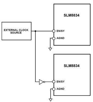
Figure 14. Multiple SLM8834 Devices Driven from a Master Clock
