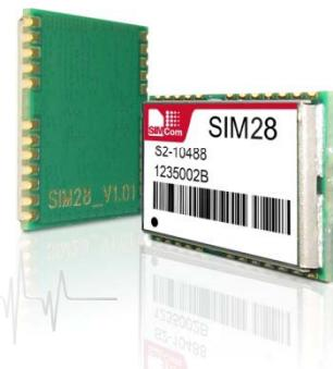
**SIMCom presents a high performance and reliable assisted GPS module-SIM28. It is in a SMT type with MTK mature GPS only navigation engine, which allows you to achieve the industry's high levels of accuracy and Time-to-First-Fix (TTFF) with lowest power consumption.**
