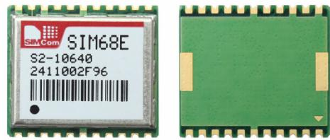
SIMCom presents a high performance and reliable GNSS module-SIM68E. This is GNSS module integrated with GPS &GLONASS system in a SMT type with MTK's high sensitivity navigation engine, which allows customer to achieve industry's high level sensitivity, accuracy, and Time-to-First-Fix (TTFF) with lower power consumption.
