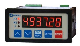
The SLIK-73 is a cross between the existing SLI-73 and SLK-73. The device has two independent counting inputs that can operate in various configurations. A programmable function input enables changing the operating mode of the counting inputs (up-down and down-up) or stopping the count. The SLIK-73 counter features an independent reset input. It has 0 or 1 relay (or OC) output with programmable activation threshold, which can be used to control external equipment.
