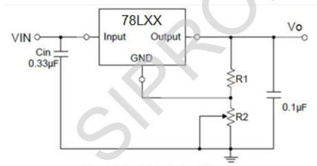
Fig.3 Adjustable Output Regulator
