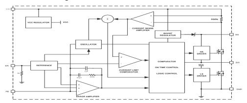
Figure 2. H9108 Block Diagram
