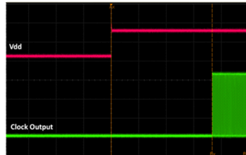
Figure 17. Startup Waveform vs. Vdd
