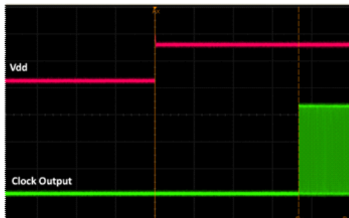
Figure 17. Startup Waveform vs. Vdd
