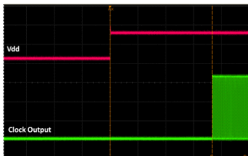
Figure 17. Startup Waveform vs. Vdd
