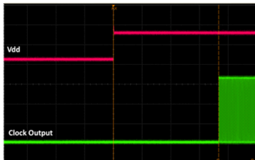
Figure 17. Startup Waveform vs. Vdd
