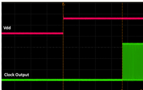
Figure 17. Startup Waveform vs. Vdd
