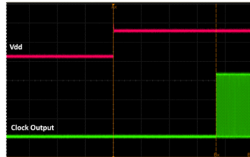
Figure 17. Startup Waveform vs. Vdd
