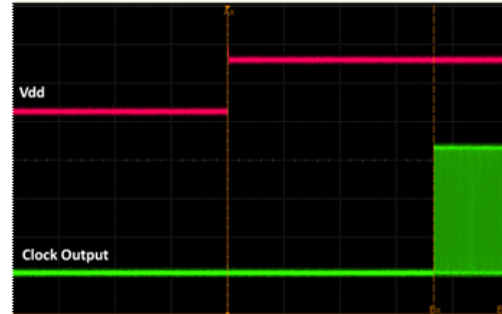
Figure 17. Startup Waveform vs. Vdd
