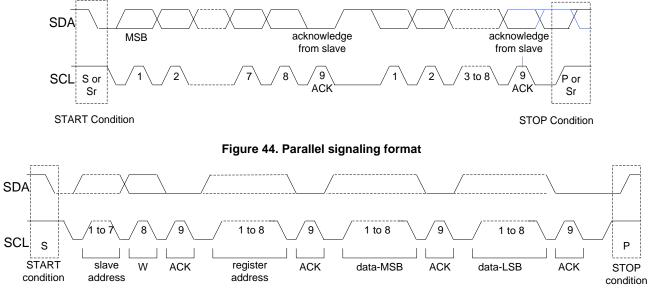
Figure 45. Parallel data byte format, write operation
