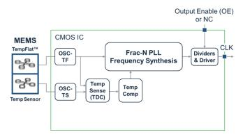
Figure 35. Block Diagram – TCXO
