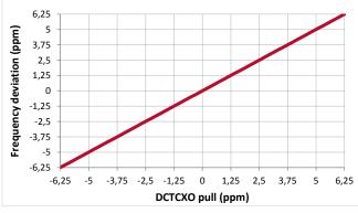
Figure 27. DCTCXO frequency pull characteristic
