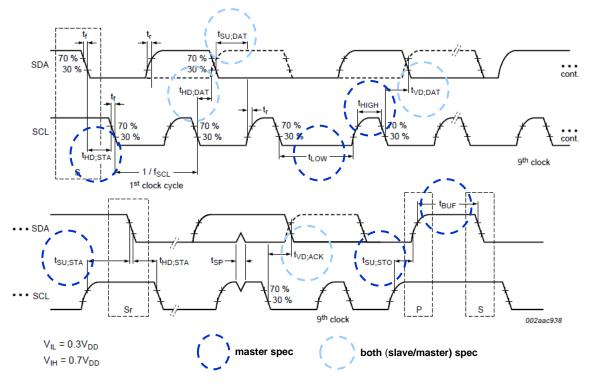
Figure 48. I<sup>2</sup>C Timing Diagram
