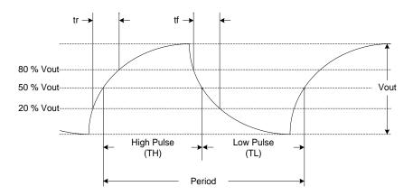
Figure 16. Clipped Sinewave Waveform Diagram<sup>[12]</sup>
