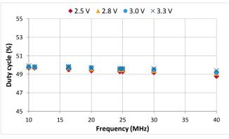
Figure 34. Duty Cycle (Clipped Sinewave)
