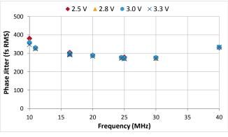
Figure 26. RMS Phase Jitter, VCTCXO (LVCMOS)
