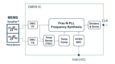
Figure 36. Block Diagram – VCTCXO
