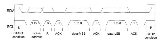
Figure 46. Parallel data byte format, read operation
