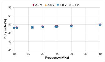
Figure 19. Duty Cycle (LVCMOS)
