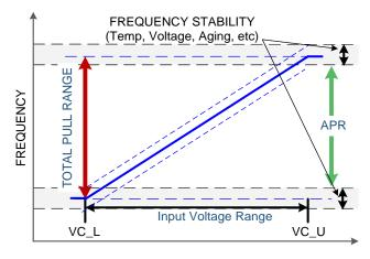
Figure 40. Typical SiTime VCTCXO FV Characteristic
