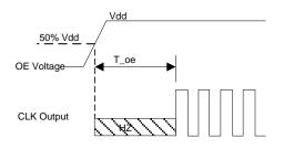
T\_oe: Time to re-enable the clock output
