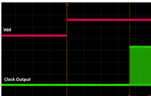
Figure 17. Startup Waveform vs. Vdd
