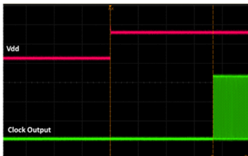
Figure 17. Startup Waveform vs. Vdd
