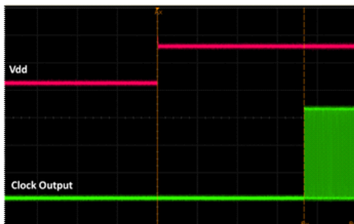
Figure 17. Startup Waveform vs. Vdd
