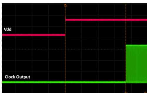
Figure 17. Startup Waveform vs. Vdd
