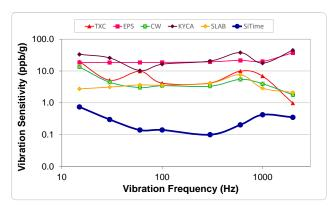
Figure 5. Vibration Robustness<sup>[5]</sup>
