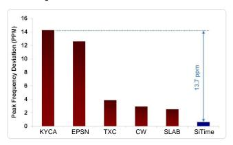
Figure 6. Shock Robustness<sup>[6]</sup>
