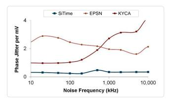
Figure 4. Power Supply Noise Rejection<sup>[4]</sup>
