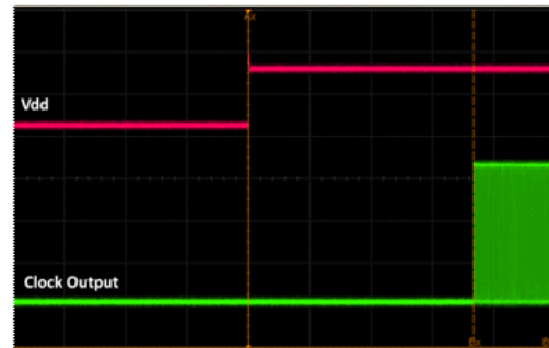
Figure 16. Startup Waveform vs. Vdd
