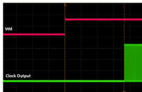
Figure 17. Startup Waveform vs. Vdd
